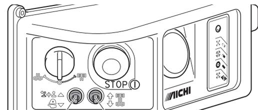
Enable Switch Lift Switch
